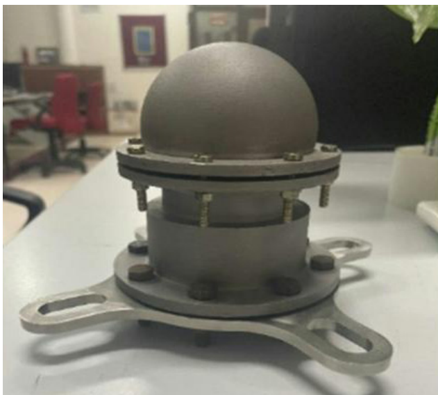
Image: AVS based Acoustics Collection System
