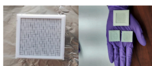
Fig 2: 3-D Printed Mold for X, Y and z-Axis
