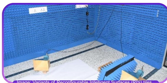
Image: Variants of Reconfigurable Intelligent Surfaces (RIS) tiles
