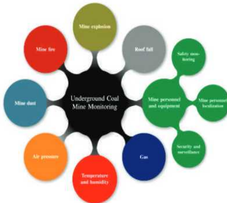
Fig. 2.5: Various parameters requiring real-time detection and monitoring through robust sensors in a hazardous and dynamic environment
