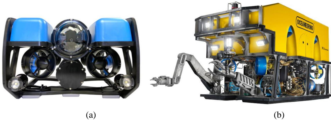
Fig. 3.6: Example of ROVs, (a) BlueROV2 from Blue Robotics and (b) Millennium Plus ROV by Oceaneering.
