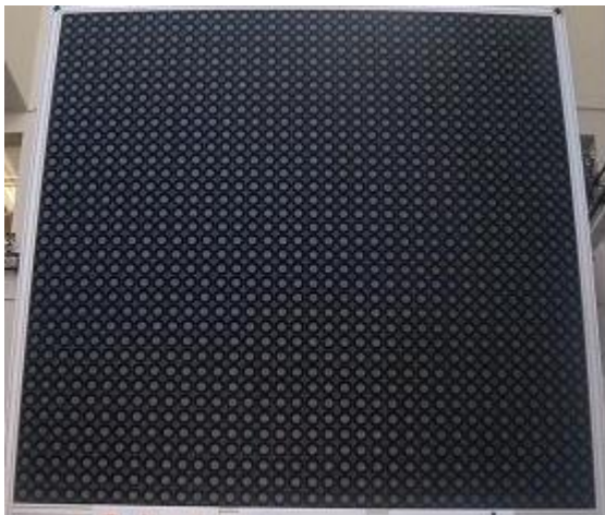
Figure 1. Typical WindShape Structure, with a 2D-array of controllable fans
