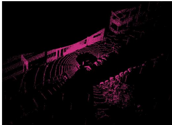
Figure 16: Example 3D point cloud data collected using 64 channel LiDAR at IIT Hyderabad
