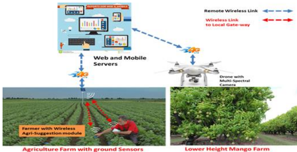
Figure 58: A system architecture for plant disease recognition using a hand-held device and server connection.
