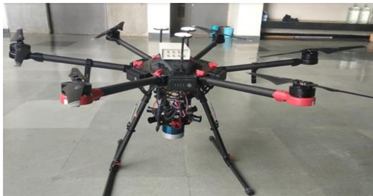
Figure 18: LiDAR sensor integrated with drone
