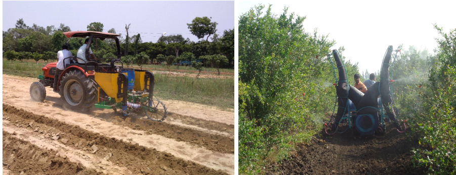
Figure 8.2: Current physical systems on tractor drawn sensor based sugarcane planter, and an ultrasonic sensor based pesticide applicator, which shall be made IoT enabled and R3 Cloud Connected to be provisioned as a Live Testbed.
